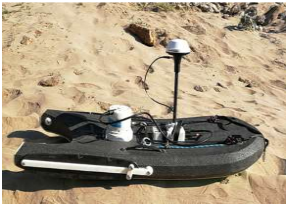
Determination of the Cross sectional area using an Acoustic Doppler Profiler (ADCP) for under water profiling
